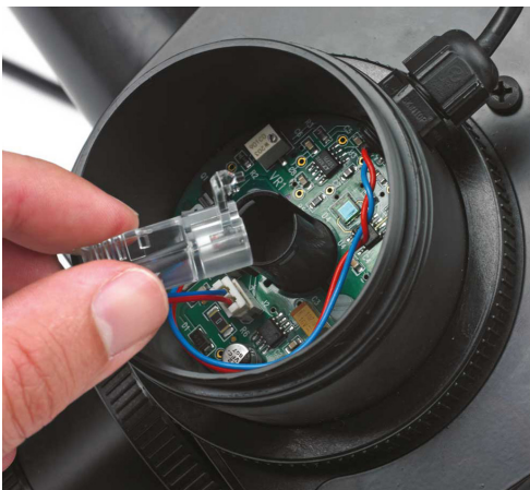
Figure 6 Replacing the light source
