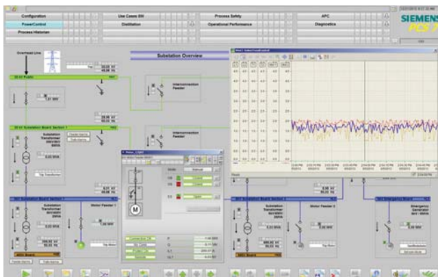
Example of a plant display for medium-voltage switchgear with trend window and faceplate of a medium-voltage motor
